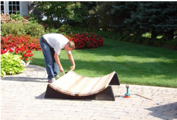
With the drain stave in the center, insert additional staves to the end of each cradle base.
